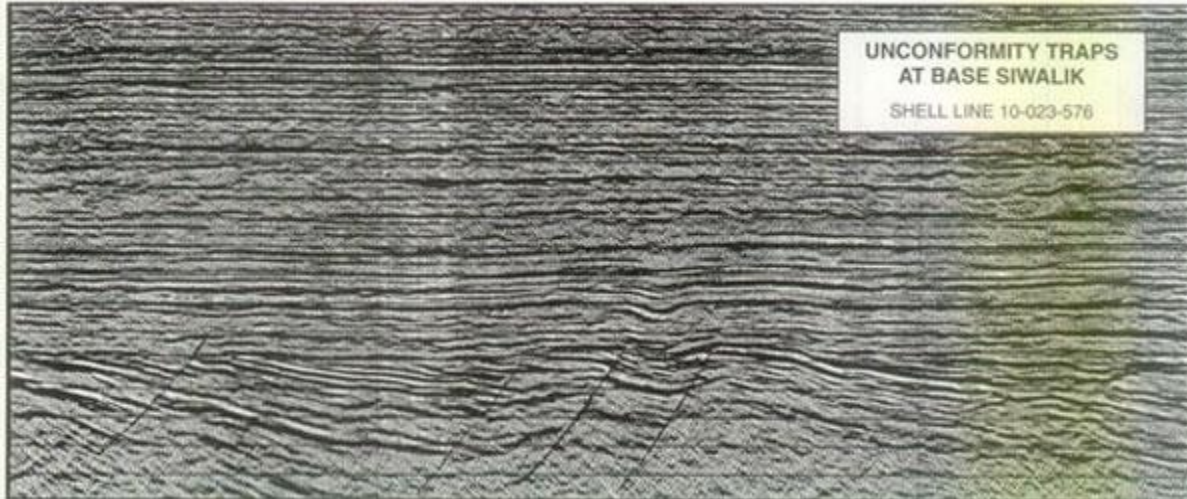
Figure 13: Seismic Expression of Unconformity Traps
